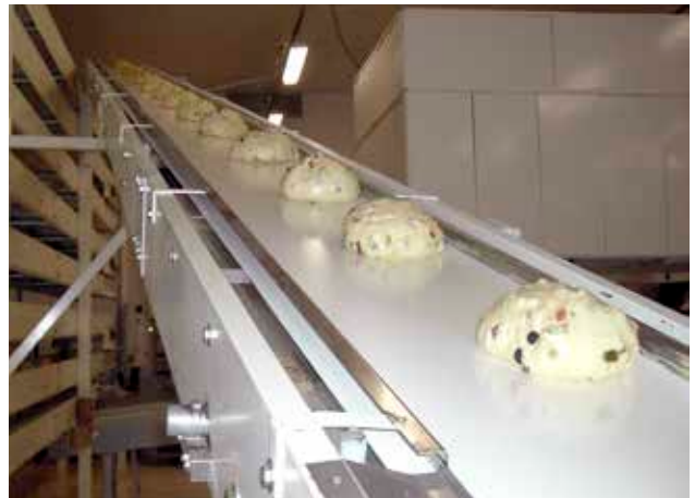
Inclined conveying towards multistory open air proofer
