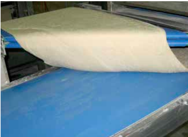
45° merge dough conveying over double fixed knife edge
