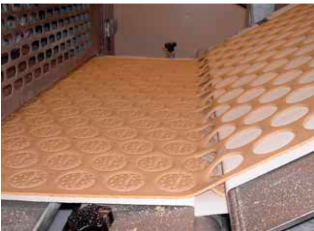
Rotary cutter and scrap return belt
