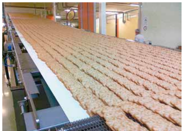
Crackers cooling conveyor
