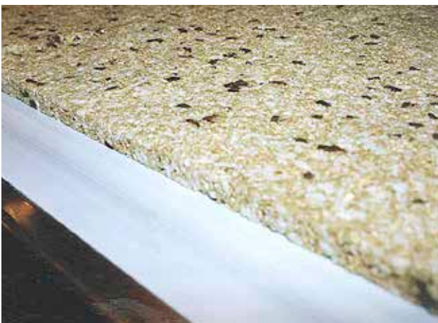
Muesli conveying on a dehesive belt
