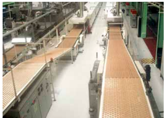
Biscuits cooling conveyor
